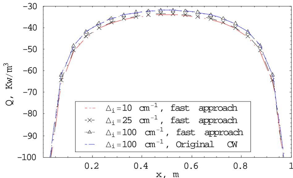
Figure 5. Radiative source term surface in two-dimensional cavity with an isothermal gas mixture at 1000 K, cold black walls. Comparison for different  $\Delta_i$  with the original CW method of solution.
