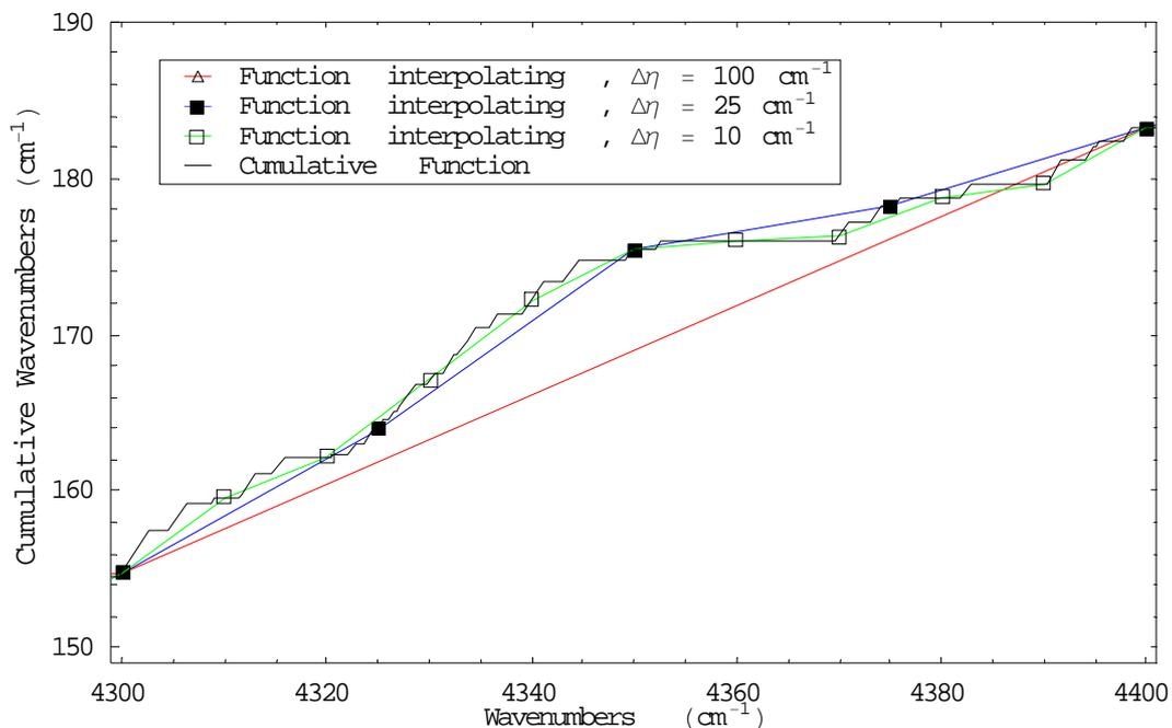
Figure 2. Comparison of Interpolating functions of CW functions distribution gray gas  $C_j = C_{14}$ ,  $\text{H}_2\text{O}$  at 2000 K.
