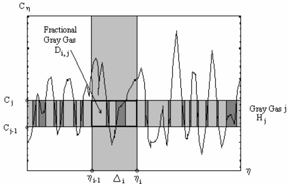
Figure 1. CW modeling by fractional gray gases.
